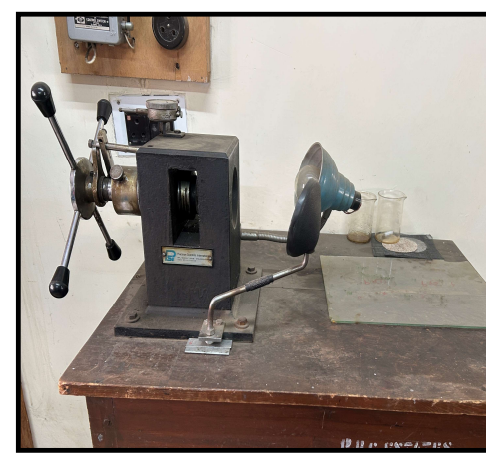
Cupping test machine
